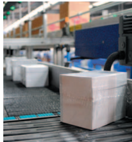
Barcodes track each individual product pack throughout the packing process.
