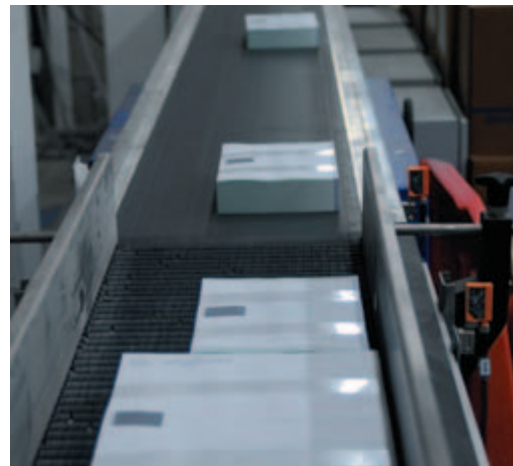
Conveyors moving finished orders from guillotine to Smartpack
