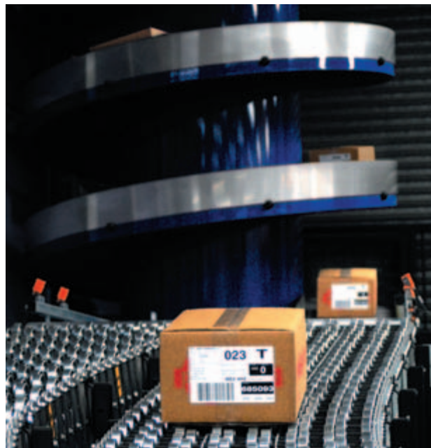
Packed product cartons leave the Smartpack system automatically labelled
