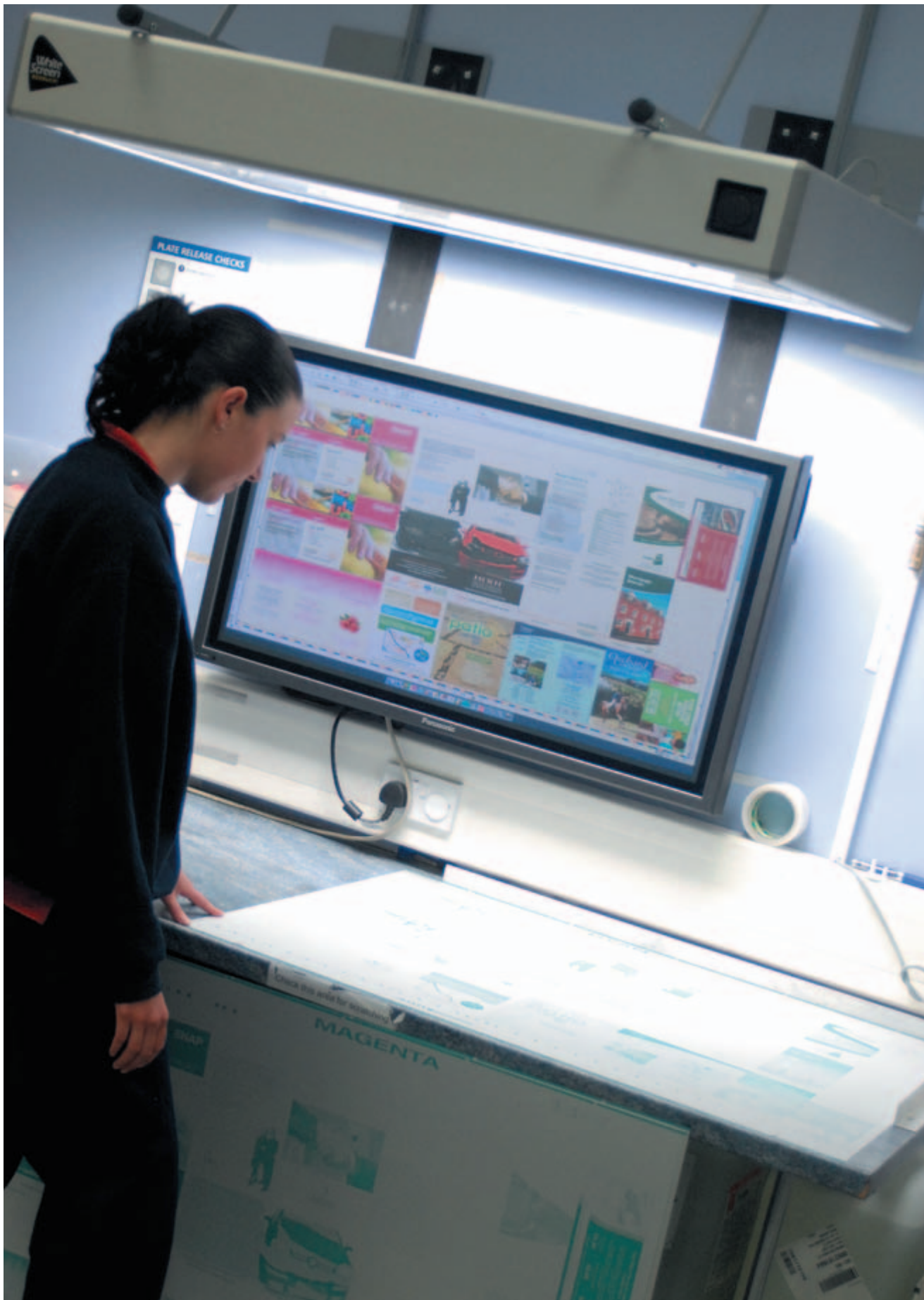
Prepress technician inspects printing plates before releasing them for production.
