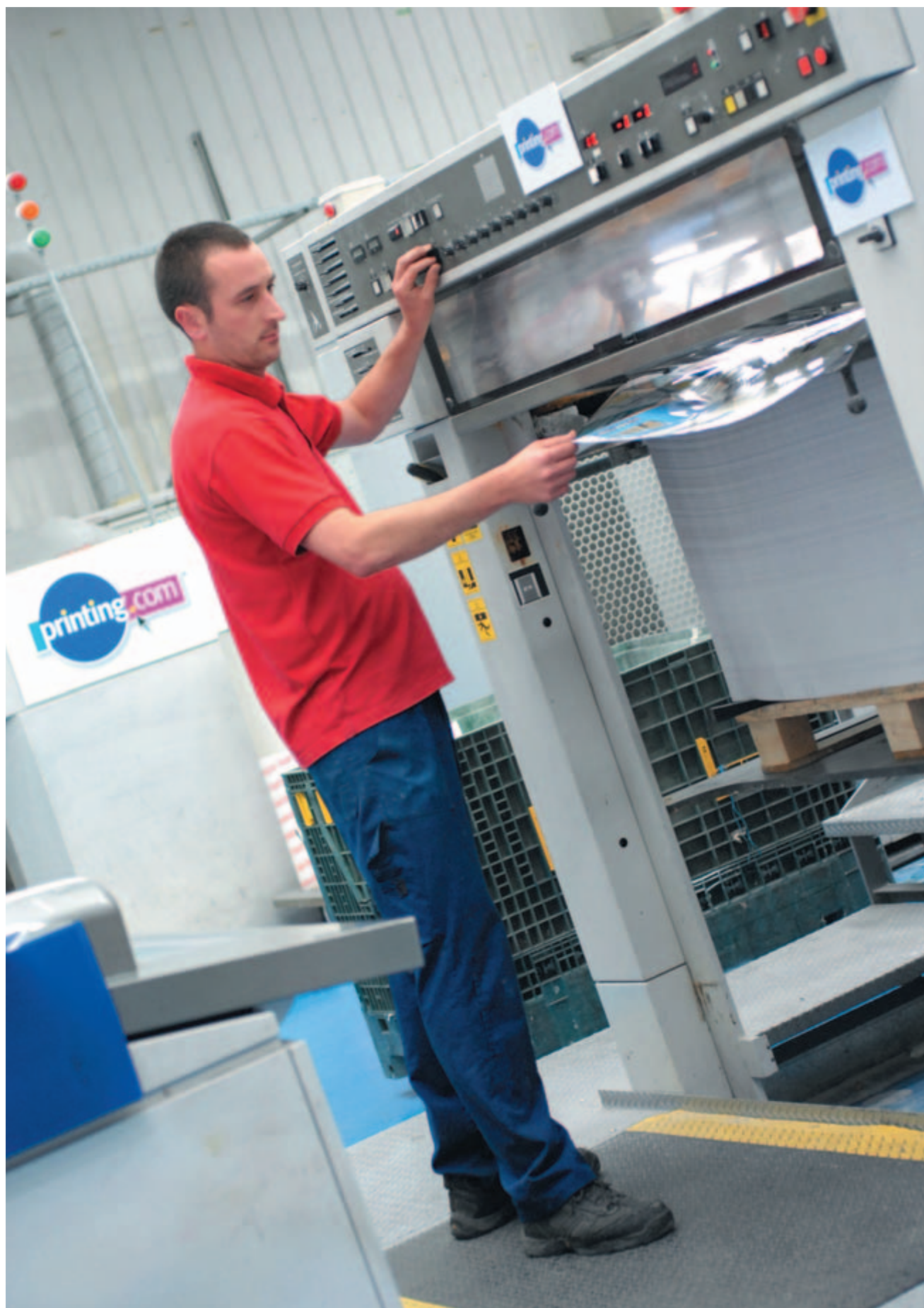
Our 'double-decker' large format Komori press prints both sides of the sheet at the same time reducing production time.
