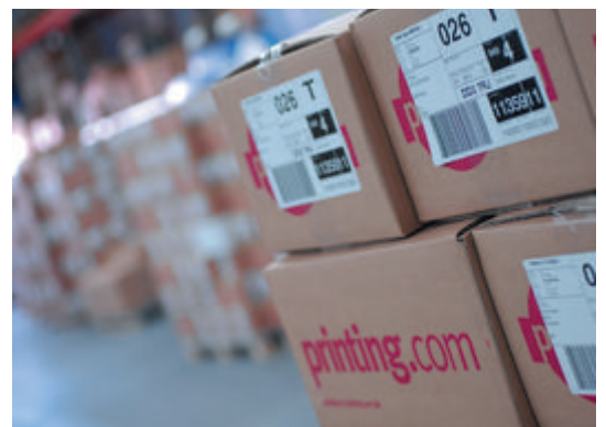
Cartons are automatically sealed and labelled before being loaded onto pallets for shipping.
